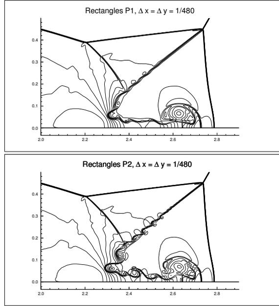
Figure 1. Euler equations of gas dynamics: Double Mach reflection problem. Isolines of the density around the double Mach stems. Linear polynomials on squares  $\Delta x = \Delta y = \frac{1}{480}$  (top); and quadratic polynomials on squares  $\Delta x = \Delta y = \frac{1}{480}$  (bottom).
