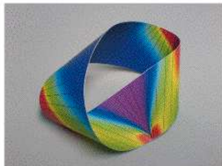
Figure 1 Photo of a paper Möbius strip of aspect ratio 2x. The strip adopts a characteristic shape. Inextensibility of the material causes the surface to be developable. Its straight generators are drawn and the colouring varies according to the bending energy density.
