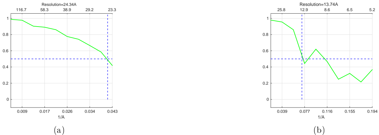
Figure 4: Fourier Shell Correlations (FSCs) for the noisy reconstructions presented in Figure 2. The FSC measures the normalized cross-correlation between the recovered 3-D structure and the (smoothed) ground truth 3-D structure over corresponding shells in Fourier space (i.e., as a function of spatial frequency). The resolution is determined as the frequency where the FSC curve drops below 0.5. This is the standard resolution measure in the cryo-EM literature. (a) FSC for the TRPV1 reconstruction, giving resolution of 24\text{\AA} ; (b) FSC for the BPTI reconstruction, giving resolution of 13\text{\AA} .
