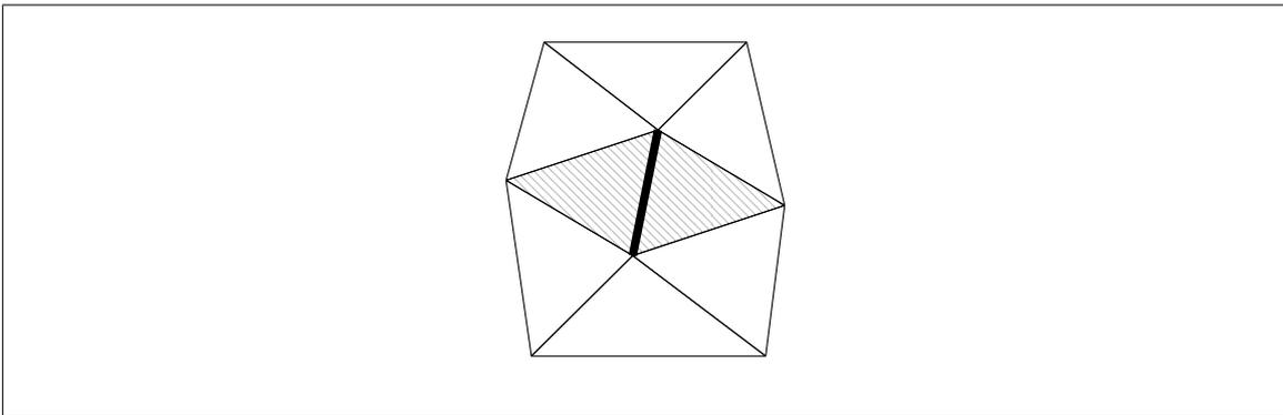
Figure II.1: Illustration of macropatch and micropatch in a triangulation. The macropatch around the thick edge segment is displayed. The hatched area indicates the micropatch of the edge.
