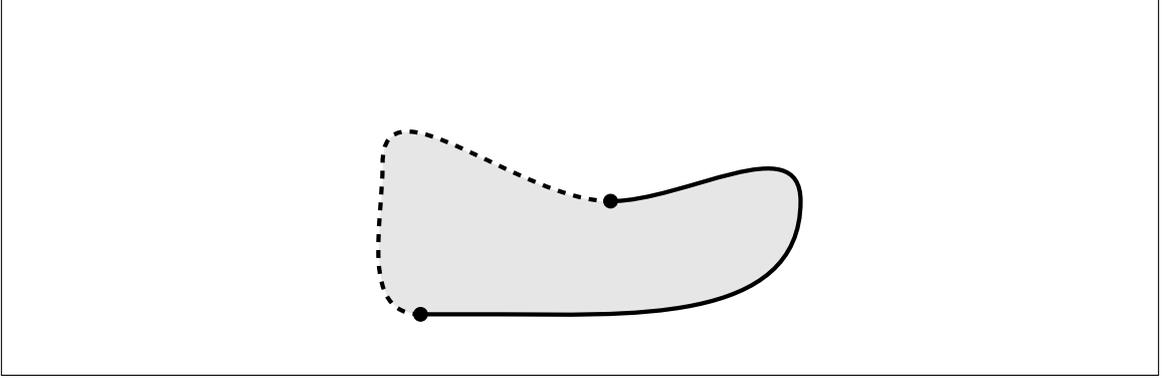
Figure VI.2: Schematic depiction of a domain  $\Omega$  (shaded area), an admissible boundary patch  $\Gamma_T$  (thick line), its complementary boundary patch  $\Gamma_N$  (dashed line), and the interface  $\Gamma_I$  (dots) between the patches.
