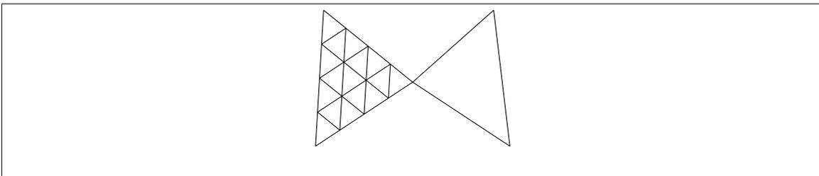
Figure II.3: Two triangles that do not triangulate a manifold. If the left triangle is subject to iterated uniform refinement, then the produced triangles do not degenerate, but the length between adjacent triangles become incomparable.
