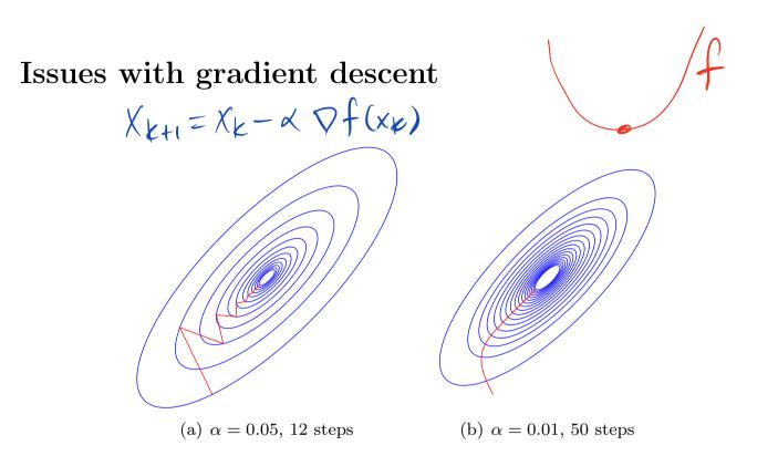
Figure 1: Gradient descent on a parabolic function with different choices of time steps. For larger time steps the iterations bounce back and forth, limiting progress towards the minimizer, while for smaller time steps the descent path is more direct.
