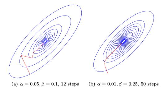
Figure 2: Heavy ball method for different choices of time step and momentum parameter. Momentum acts to average out the descent direction in time, limiting the bouncing effect for larger time steps. Momentum builds up speed and makes more progress towards the minimizer in the same number of steps as gradient descent.
