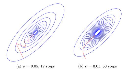
Figure 3: Gradient descent on a parabolic function with different choices of time steps. For larger time steps the iterations bounce back and forth, limiting progress towards the minimizer, while for smaller time steps the descent path is more direct.
