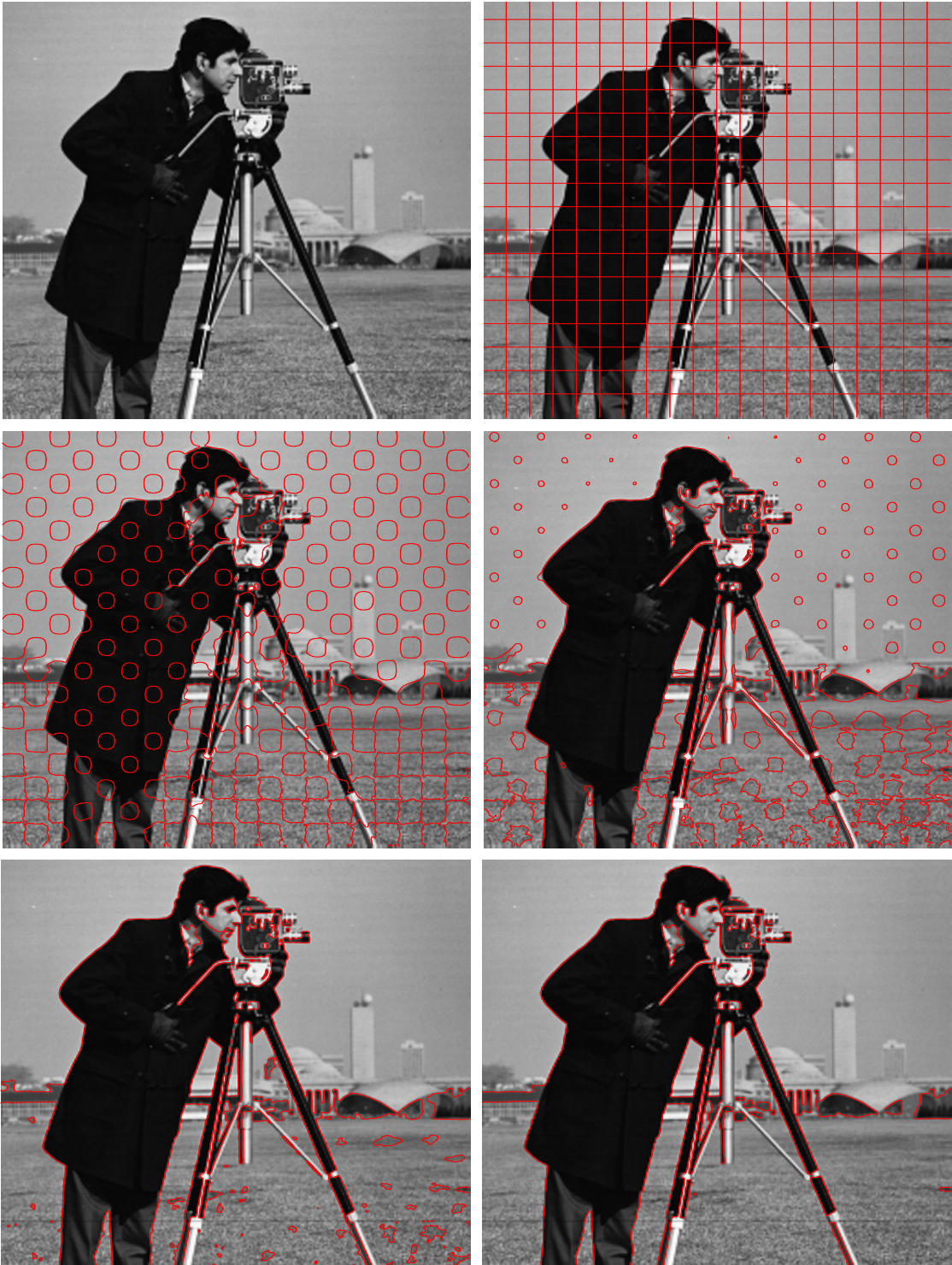
Figure 9: Illustration of gradient descent for segmenting the cameraman image. Top left is the original image, and top right is the initialization of the gradient descent algorithm. The lower four images show the evolution of the zero level set of u .
