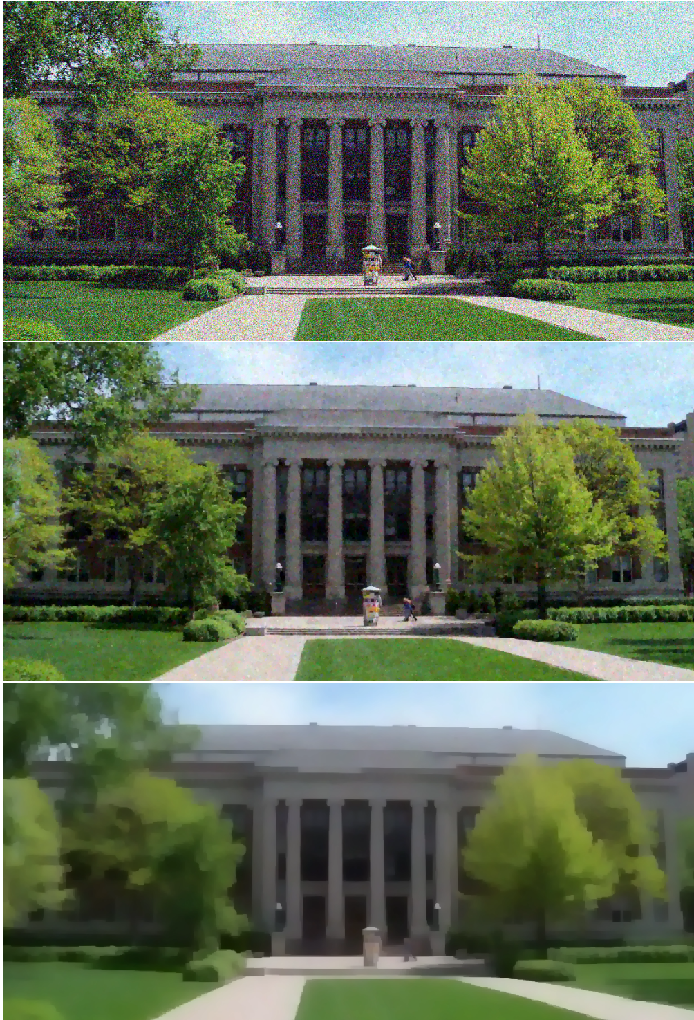
Figure 8: Example of TV image restoration: (top) noisy image (middle) TV restoration with small value for \lambda , and (bottom) TV restoration with large value for \lambda .
