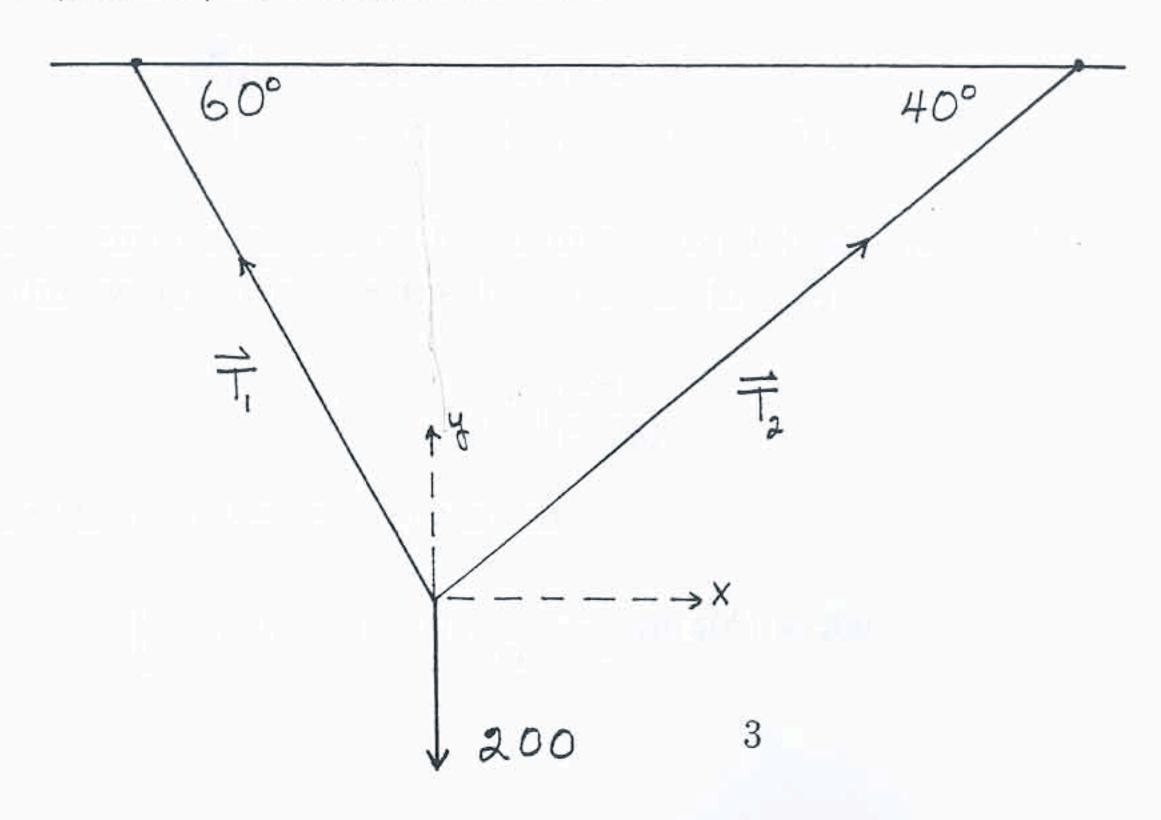
Solution. The first thing we must do is to decide on a coordinate system. As indicated in the above diagram we place the origin of the coordinate system on the object. We place the x axis parallel to the ground and the y axis vertical. In this coordinate system we can easily specify the direction of all forces. The two things that we do not know are the magnitudes of the forces  $\vec{T}_1$  and  $\vec{T}_2$ . From the given geometry we easily see that
