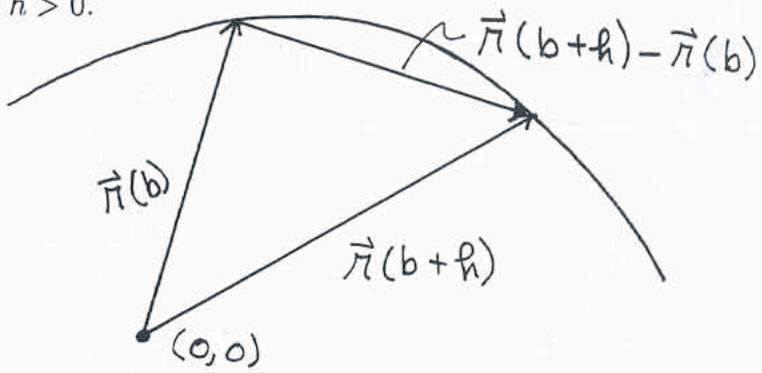
The vector  $\vec{r}(b+h) - \vec{r}(b)$  is a secant line or chord for the curve  $\vec{r}(t)$ . The number h is a scalar and so 1/h is a scalar. The vector  $\frac{1}{h}[\vec{r}(b+h) - \vec{r}(b)]$  is a vector with initial point the point located by  $\vec{r}(b)$ . It is parallel to the vector (chord)  $\vec{r}(b+h) - \vec{r}(b)$ . Suppose  $\vec{r}'(b)$  exists. It follows that
