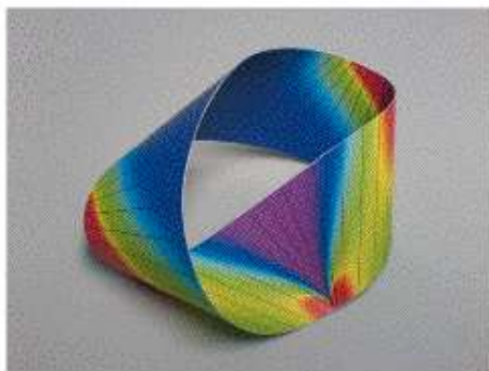
Figure 1 Photo of a paper Möbius strip of aspect ratio 2\pi . The strip adopts a characteristic shape. Inextensibility of the material causes the surface to be developable. Its straight generators are drawn and the colouring varies according to the bending energy density.
