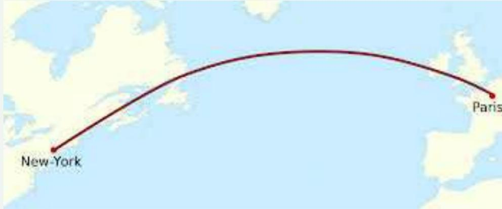
The shortest path between two points on a curved surface is a **geodesic arc**.
