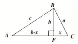
By definition, F is the foot of the altitude (perpendicular) drawn from B to AC. As usual, a, b and c denote the lengths of the sides opposite the vertices A, B, and C respectively. We define x to be the distance from C to F: positive in case F is in the ray CA and negative if not. (We would get a negative value if we had an obtuse angle at C.) Similarly, b - x is the distance (with  $\pm$  sign) from A to F.
