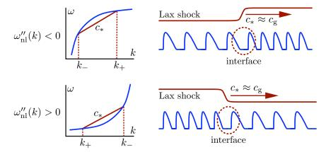
FIGURE 1.3. The relation between concave (top) and convex (bottom) dispersion relations and the resulting weak shock profiles is illustrated. The velocity  $c_*$  of the interface, given by the Rankine–Hugoniot condition (1.13) and therefore by the slopes labelled  $c_*$  in the insets, is close to the group velocity  $c_{\rm g} = \omega'_{\rm nl}$ , which is positive for the dispersion relations shown to the left.
